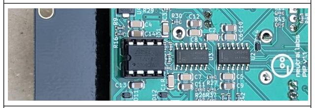
Put the ATTiny85 IC in the U1 socket as shown. You may have to bend its legs inward slightly. The notch in the IC must match the notch in the socket and the notch in the line on the PCB!
