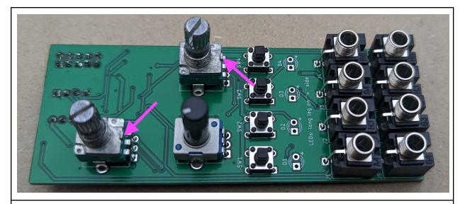
Snip off the little anti-rotation tabs near the bottom of RV1 and RV2 with a wirecutter. Put RV1, RV2, RV3 and J1 to J8 in their places as shown. **Do not solder yet!**
