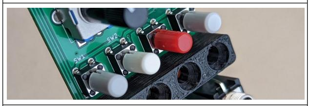
Add the button caps as shown: Gray on SW1 and SW4, white on SW2 and red on SW3. Press down on them firmly until they stay in place by themselves. Make sure they point up perpendicular to the PCB.
