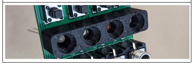
Now put the LED holder over the LEDs as shown. The wide cut in the holes should be facing up, towards you. The holder is there to keep the LEDs in position and minimize light bleed from each LED to neighboring light ports on the front panel.
