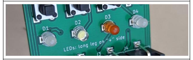
Now insert the LEDs in their holes without soldering them. D1 and D4 are the milky LEDs with longer legs. D2 is a clear white LED with shorter legs. D3 is an orange LED identifiable by, you may have guessed it, its orange color. The long legs of the LEDs go on the side marked on the PCB with a "+"!
