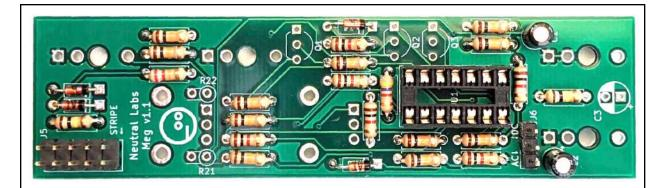
Add the 2x5 pin power header (J5) and the 3-pin header (J6). As with the IC socket, it's best to solder a single pin first. You may want to hold the headers in place with a piece of sticky tape while soldering. Another trick is to plug the Eurorack power cable into the header before and hold it this way.
