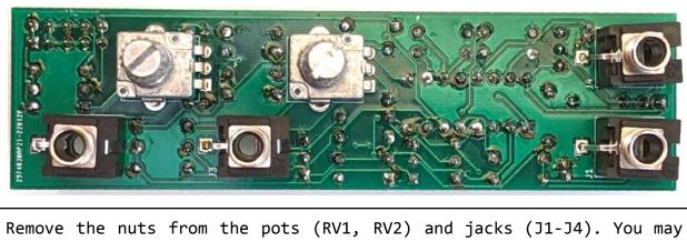
want to clip the little silver anti-rotation tag off the pots with a wirecutter. Fit the pots and jacks onto the PCB without soldering yet. Then put on the front panel. Add and lightly tighten all the nuts to hold the panel in place. Carefully flip everything back over and solder.
