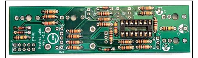
Next, put in the IC socket (U1). It has a little notch on one side which should match the notch of the white outline on the PCB. (It's not harmful if you put one in the other way around by accident, as long as you make sure the IC is facing the right way when you plug it in later.)
