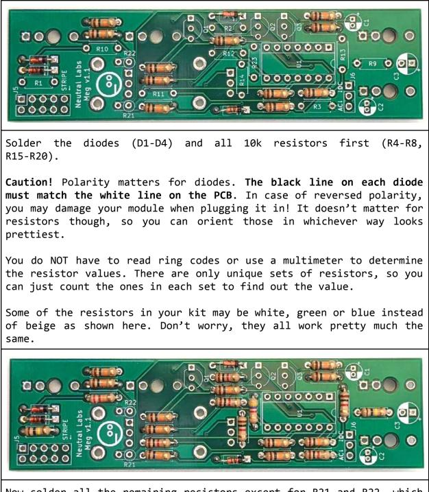
Now solder all the remaining resistors except for R21 and R22, which will get a special treatment later on.
