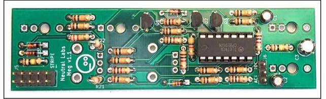
Now on to C3 (pay attention to the polarity) as well as the 3 transistors Q1, Q2 and Q3. Again, polarity matters for the transistors. Insert them facing them as the outline on the PCB indicates. Make sure that the transistors labeled J109 go into Q1 and Q2 and the 2N3904 goes into Q3. They're very different beasts and not interchangeable!
