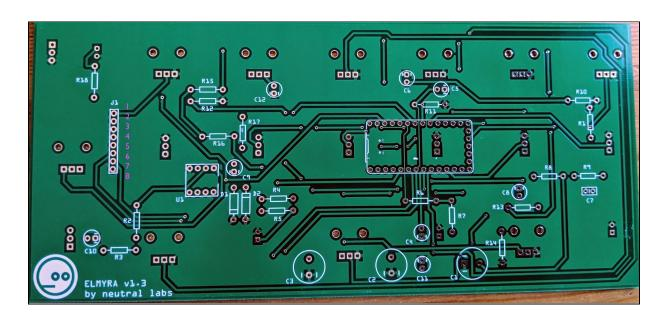
(D are diodes, R are resistors, C are capacitors, U are the potentiometers as well as the IC and its DIP8 socket, S are switches and LED are, you might have guessed it, LEDs.)
