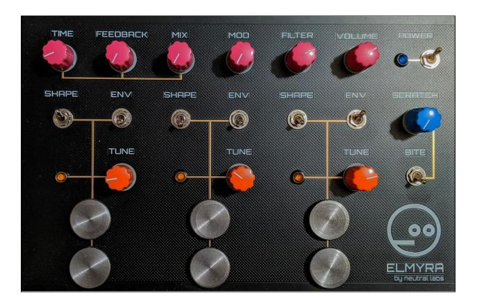
Now put in the 6 touchpads. You must use the plastic washers under the touchpads on the top side! On the bottom side, tighten the nut and do not use any washers. The nut must be in contact with the metal film below.
