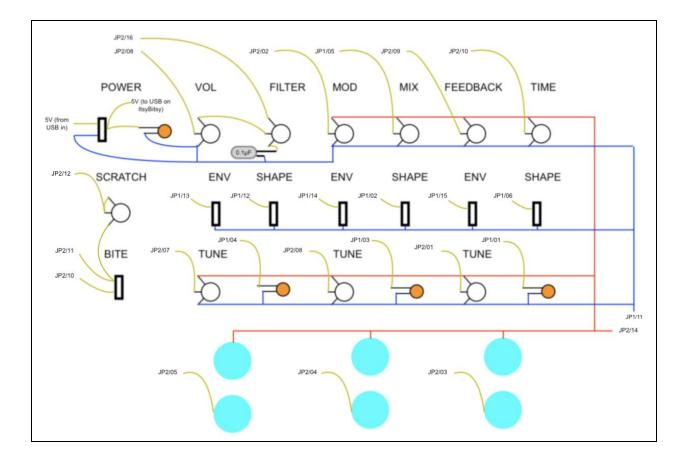
Connect wires as shown. First solder the blue and red strands of wire to their pins. You don't need to run individual wires, just use a single one for each colour per row and remove the insulation right where the solder points are.
