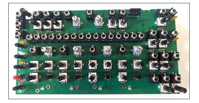
The orange LEDs go into D9-D10, D39, D40. The red one goes into D42 and the green one into D41. The 4-legged RGB LED goes into D43. One of its legs is longer than the others, that one goes into the hole marked with a "+". The 4 clear LEDs are a super bright orange type used to light up your fingers from below the touchpads, and they go into the 4 LED footprints at the bottom of the PCB. **Do not solder anything yet!**
