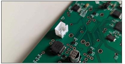
Only the desktop version has an XH connector for USB power (J4). Put it in place and solder. Double check the orientation! The open slot goes on the side towards the middle of the PCB, as indicated the on silkscreen print.
