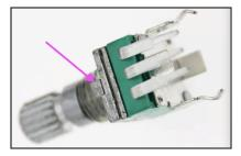
Snip off the little anti-rotation tabs near the bottom of RV1 to RV6 with a wirecutter (these are the green metal pots).
