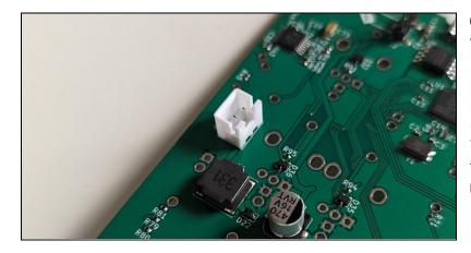
Only the desktop version has an XH connector for USB power (J4). Put it in place and solder. Double check the orientation! The open slot goes on the side towards the middle of the PCB, as indicated the on silkscreen print.
