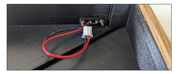
Now plug in and test your module. For the Eurorack version, use the provided Eurorack power cable. For the desktop version, insert the XH cable from the case into the XH header (J4) on the back of the module, and power the case via the USB-A-to-USB-C cable.
