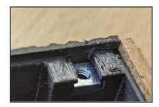
For the Eurorack version, place your new module in a rack. For the desktop version, insert the 4 square nuts into the 4 slots in the corners of the case. Put the module on top and secure it with the 4 black hex screws, or any other M3 screws (such as those commonly used for Eurorack).
