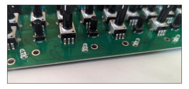
Attach and tighten all the Thonkiconn socket nuts, or at least those that are close to any LEDs and the 5-pin headers (J5-J6). This ensures a constant distance between PCB and front panel which is important for soldering the LEDs and 5-pin headers.
