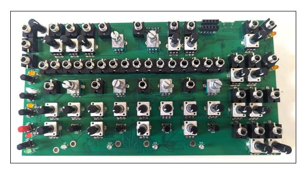
The orange LEDs go into D9-D10, D39, D40. The red one goes into D42 and the green one into D41. The 4-legged RGB LED goes into D43. One of its legs is longer than the others, that one goes into the hole marked with a "+". The 4 clear LEDs are a super bright orange type used to light up your fingers from below the touchpads, and they go into the 4 LED footprints at the bottom of the PCB. **Do not solder anything yet!**
