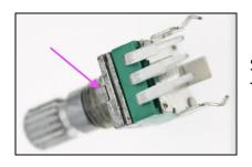
Snip off the little anti-rotation tabs near the bottom of RV1 to RV6 with a wirecutter (these are the green metal pots).
